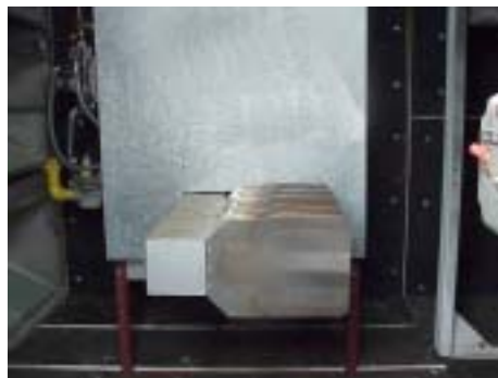
Side View of Minnox Burner in Duct.
