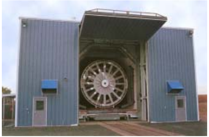
Arrow Tank's Heat Treatment Furnace uses natural gas as its primary fuel and propane as a standby fuel.
