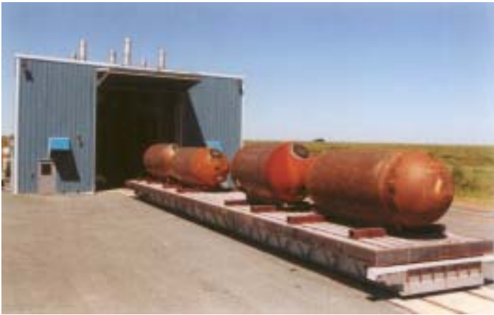
Arrow Tank's Heat Treatment Furnace uses natural gas as its primary fuel and propane as a standby fuel.
